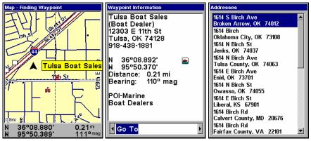
Map Page showing location of the address on the map, highlighted by cursor (left). This address is a business in the POI database, so you can display the POI information window, then navigate to it (center). This address is not in the POI database (right), so the Waypoint key will not display any information for this address.
